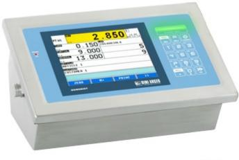
Weight indicator with a big touch screen display, for ATEX 2 & 22 areas classified at risk of explosion. Protection methods according to ATEX II 3G Ex nR IIB T6 Gc X for gases ATEX II 3D Ex tc IIIC T85°C Dc IP68 X for dust. Suitable for advanced industrial applications, it's fitted with 3 serial ports, configurable printouts and integrated alibi memory. CE-M approvable (OIML R-76 / EN 45501).
